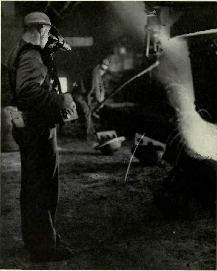
One of many quality controls—an optical pyrometer records temperature of steel pouring into ingot molds.
